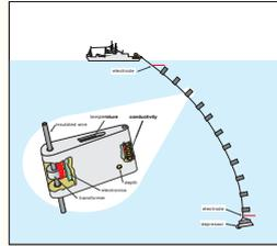
The towed CTD-chain enables high resolution measurements of the upper ocean underway. Fins equipped with temperature, conductivity and pressure sensors are inductively coupled to a simple coated steel wire. During both cruises 86 sensor fins were attached 3 m apart to a 260 m long wire. The chain was towed with about 6 knots.
